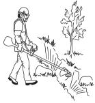
5 Keep a good balance and a firm foothold. Do not overreach. Keep proper footing and balance at all times. 6 Always hold the machine with both hands. Hold the machine on the right side of your body.
