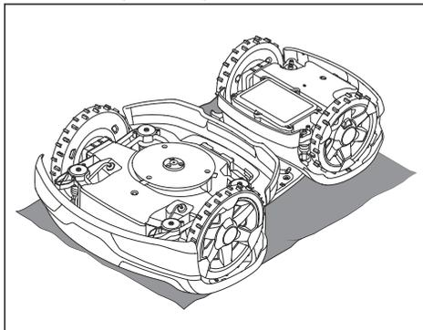
3. Remove the 6 screws and remove the battery cover.
