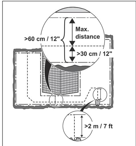
**Note:** Make sure that the guide wire has as much free area as possible to the left of the guide wire when facing the charging station. Minimum distance between the guide wire and boundary wire is 30 cm / 12 in.
