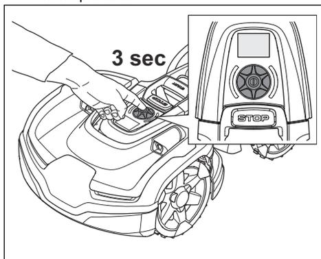
**Note:** Make sure that the **STOP** button is pushed down. If the **STOP** button is not pushed down a **STOP** symbol will show on the display.
