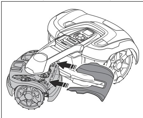
2. Put the top cover in position (A) and push the 2 magnets to assemble the top cover (B).
