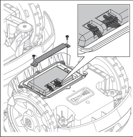
5. Disconnect the two cables from the battery and remove the battery.
