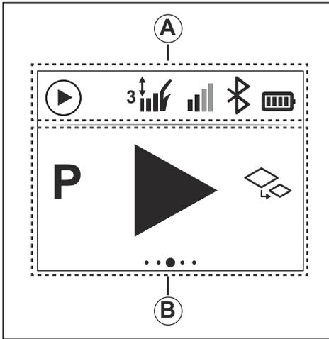
The display shows the status bar and the main menu symbols. If an error occurs, the display shows an error indication. Refer to *Error icons in the Automower® Access display on page 46*.
