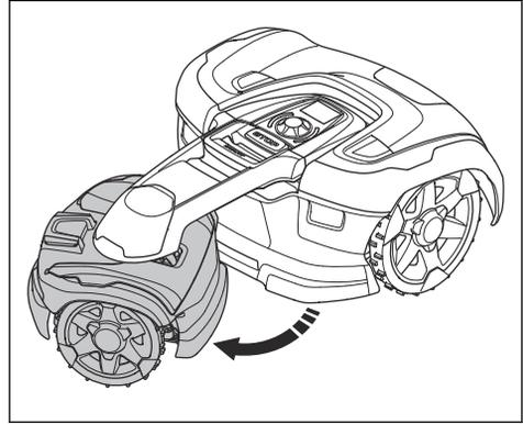
3. Put a protection between the rear top cover and the link arm. This is to prevent damage to the rear top cover.
