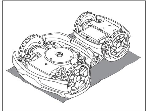
4. Rotate the skid plate so that its holes align with the screws for the blade.
