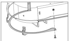
Position the mulch baffles to the underside of the deck and secure loosely with the nuts.
