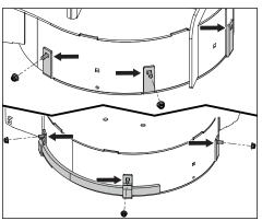
Loosely install the mulch cover to the deck and the previously installed right mulch baffle and right debris baffle with the nuts and bolts.
