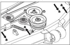
Loosely install the debris baffles to the deck and the previously installed mulch baffles with the nuts and bolts.
