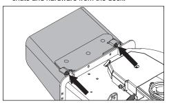
Raise and support the mower. Remove and retain the existing blade bolts and cutting blades.
