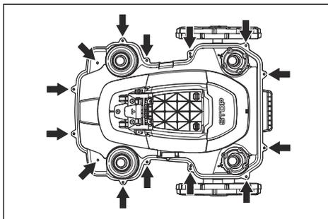
5. Lift the rear edge of the top section of the chassis.
