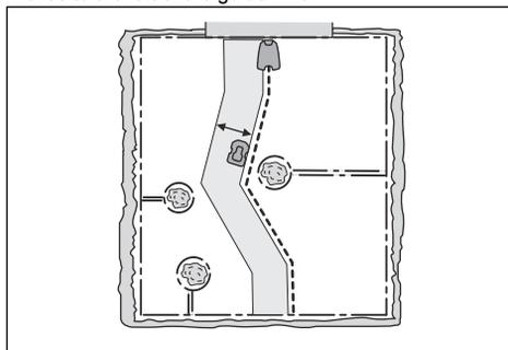
The corridor width is adjusted automatically. If it is necessary to adjust the corridor width manually for the product to operate satisfactorily, you can set the corridor width between 0-9. If guide corridor width is set to 0, the product straddles the guide wire. The factory setting is 6 for the boundary wire and 9 for the guide wire.
