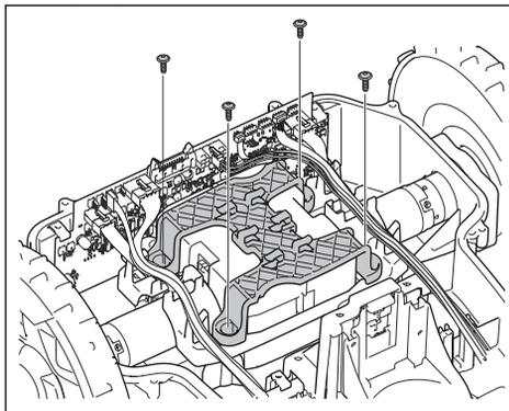
9. Disconnect the battery connection from the main circuit board.
