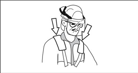
5. Adjust the harness until the cutting attachment is parallel to the ground.
