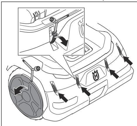
2. Remove the wheel cover with the flat screwdriver on the Combi tool.
