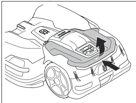
2. Loosen the clips with the flat screwdriver on the Combi tool and remove the rear bumper.
