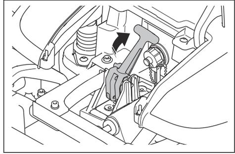
13. Install the center top cover on the cutting deck.
