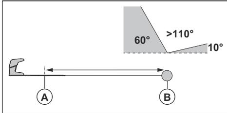
**Note:** Short reversing distance decreases the risk of track marks. A long reversing distance can be necessary to have good satellite signals at the docking point.
