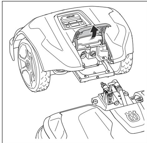
4. Remove the center top cover on the cutting deck.
