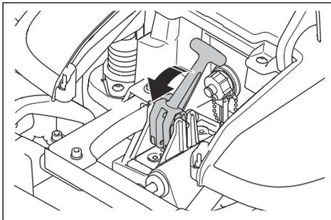
4. Push down the lever and lift up the front of the cutting deck by the handle. Make sure that the cutting deck is in a vertical position.
