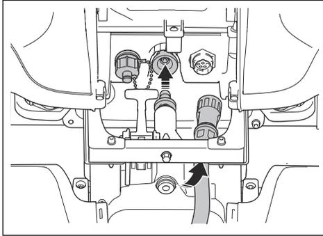
7. Align the shaft with the hole in the frame.
