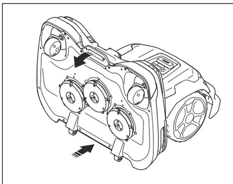
2. Lift the rear part of the cutting deck and tilt the lever.
