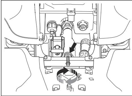
8. Install the screw with the ratchet wrench or torque wrench, 10mm. Tightening torque 5 Nm.
