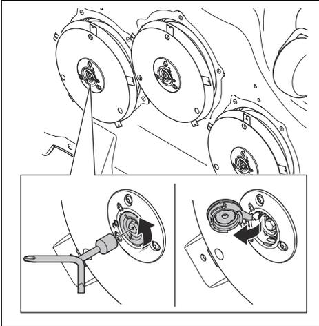
5. Loosen the screw with the Combi tool.
