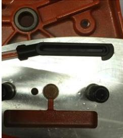
The new crankcase has a new slot in the bar pad area and the new chain guide plate has a slot that is adapted to the new oil pressure hose.
