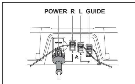
3. Switch the connections between the guide wire and the boundary wire in the charging station.
