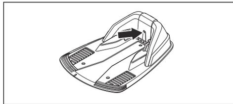
2. Check that the boundary wire connections to the charging station are properly connected and not damaged. Check that the indicator lamp in the charging station is still flashing blue.
