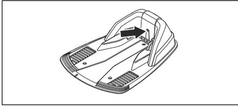
2. If the indicator LED lamp does not have a green light, do a check of the installation. Refer to *Indicator lamp in the charging station on page 35* and *To install the charging station on page 18*.
