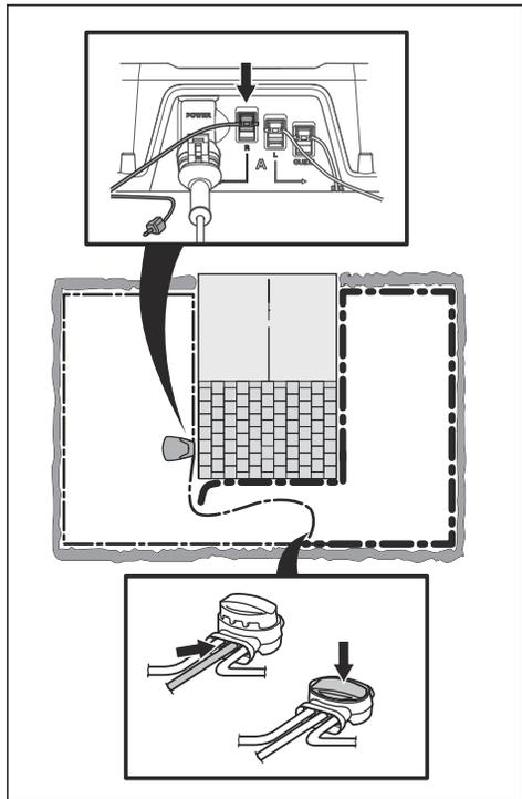
If the indicator lamp now is flashing yellow, then the break is somewhere in the wire between the disconnected end to the point where the new wire is connected (thick black line below). In that case, move the connection for the new wire closer to the disconnected end (roughly at the middle of the suspected wire section) and check again if the indicator lamp is green.
