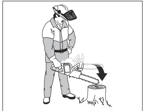
5. Make sure that the chain brake engages as the guide bar hits the stump.
