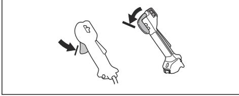
2. Press the throttle trigger lockout (A). Make sure that the throttle trigger (B) is released.
