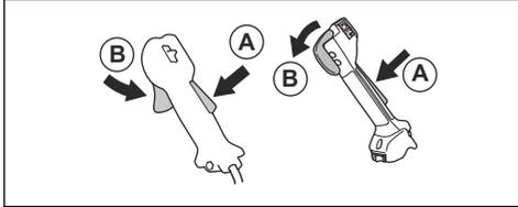
3. Release the handle and make sure that the throttle trigger lockout (A) and the throttle trigger (B) go back to their initial positions.
