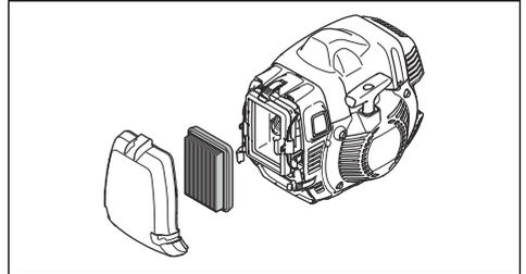
7. Close the 2 hooks and make sure that they hold the filter correctly.
