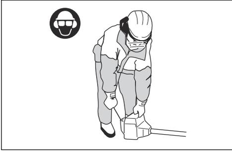
4. Pull the starter rope handle slowly until you feel some resistance, then pull the starter rope handle with force.
