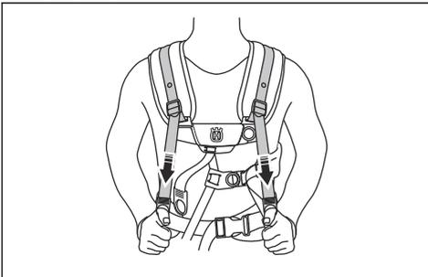
11. Adjust the side straps around the rib cage until the breastplate is aligned with the center of your chest.
