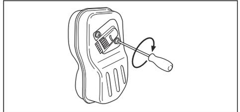
4. If the muffler on your product has a spark arrester screen, do a visual check.
