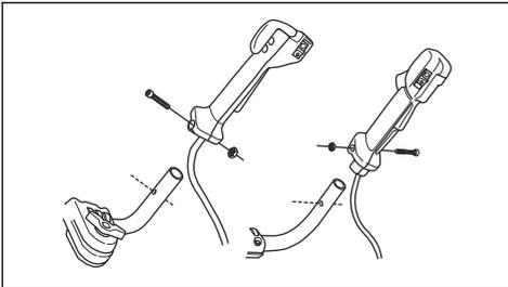
3. Align the screw hole in the throttle handle with the hole in the handlebar.
