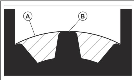
5. If the grease level is too low fill the bevel gear with Husqvarna bevel gear grease. Fill slowly and turn the drive shaft as you apply the bevel gear grease, stop at the correct level (B).
