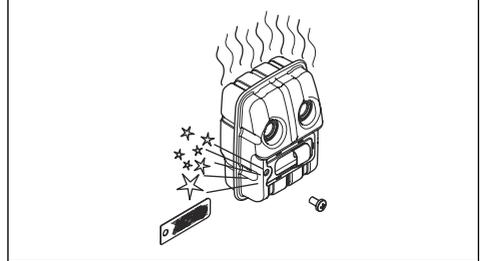
4. Clean the spark arrester mesh if it is blocked or replace it if it is damaged.
