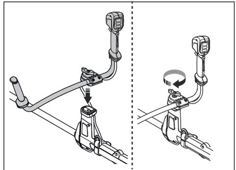
2. Attach the knob but do not tighten fully.
