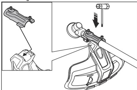
2. Attach the trimmer guard to the plate holder.
