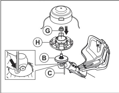
6. Install the line chute and the trimmer head cover (F).
