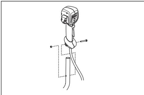
3. Align the screw hole in the handle with the screw hole in the handlebar.
