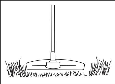
2. Do not push the trimmer head to the ground. The ground and the product can be damaged.
