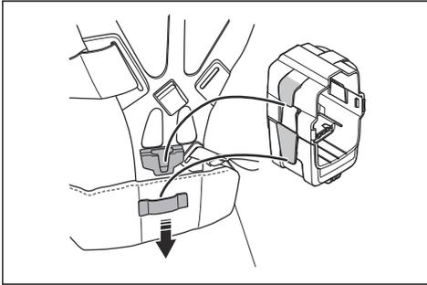
**Note:** It is possible to attach 1 extra battery to the battery carrier. The battery carrier is available as an accessory.
