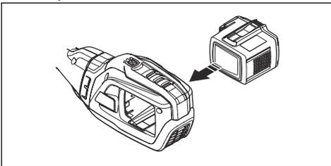
3. Make sure the battery is installed correctly.
