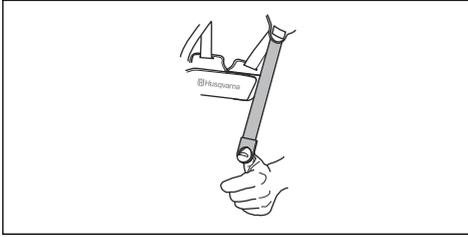
6. Adjust the height of the suspension point. For forestry clearing, the correct height of the suspension is approximately 10 cm below your hip. Refer to *Correct balance of the product on page 18*.
