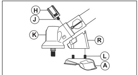
2. Remove the 2 bolts (J) on the gear housing (K). Remove the holder (R) and the bracket (H).
