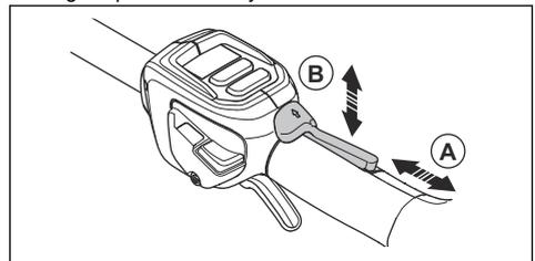
3. Make sure that the power trigger and the power trigger lockout moves freely and that the return springs operate properly.
