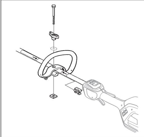
2. Move the spacer into the slot of the loop handle.
