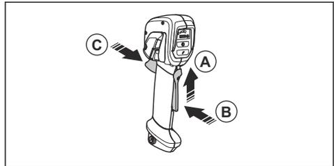
1. Make sure that the power trigger is locked when the lock is in its initial position.
