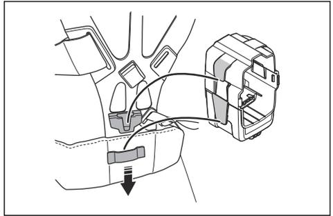
**Note:** It is possible to attach 1 extra battery to the battery carrier. The battery carrier is available as an accessory.
