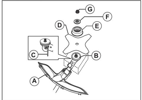
5. Make sure that the drive disc and support flange engages correctly in the center hole of the grass blade.
