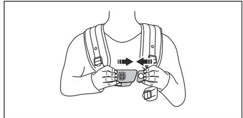
4. If the harness has a hip pad and a hip strap, make sure that the quick release function operates correctly.
