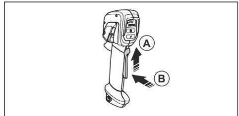
3. Make sure that the power trigger and the lock moves freely and that the return spring operates correctly.
