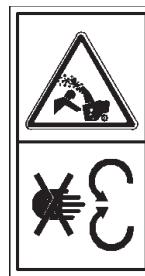
Turn the engine off before cleaning auger housing or discharge chute. Never put your foot or hand in the auger or in the discharge chute when the snow thrower is running.
