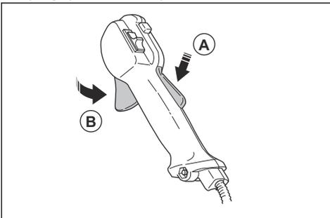
2. Push down the throttle trigger lockout and make sure that it goes back to its initial position when you release it.
