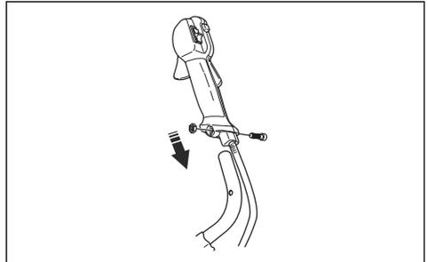
2. Install the throttle handle to the right handlebar.
