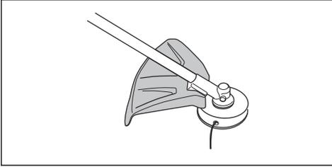
3. Replace the cutting attachment guard if it is damaged.
