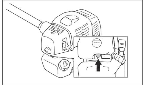
3. Move the choke control to the choke position.
