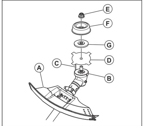
3. Turn the output shaft until 1 of the holes in the drive disc aligns with the related hole in the gear housing.
