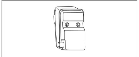
Regularly check that the muffler is securely attached to the product.
