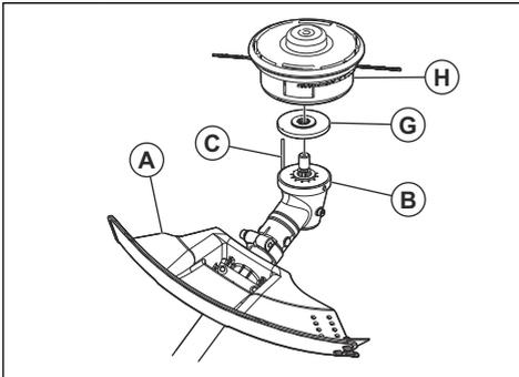
3. Turn the output shaft until the hole in the drive disc aligns with the hole in the gear housing.
