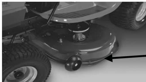
Stamped Deck Shell below, NOT reinforced
