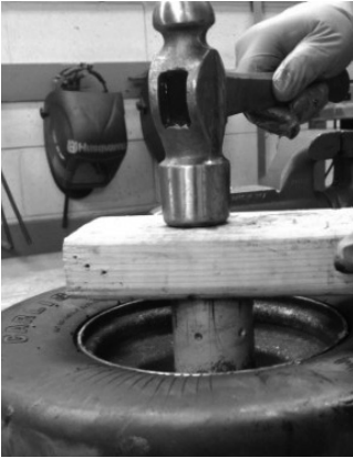
NEW SEAL INSTALLED
